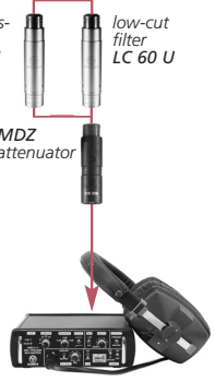
VMS 5 U: microphone pre-amplifier with MIS matrix
