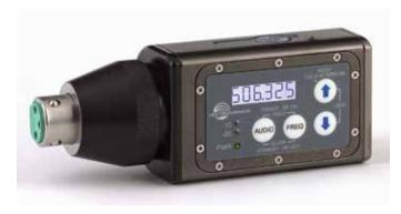
This unique plug-on transmitter design will ideally match any microphone or line level source via a standard XLR connector. Phantom power is selectable at 5, 15 and 48 volts, or can be turned off for use with dynamic microphones and line level signal sources.
