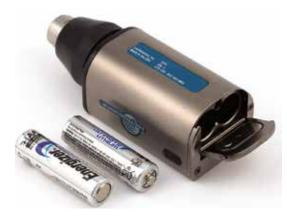
The battery compartment door is hinged to the housing and remains attached to the transmitter when opened. It latches securely in place and applies pressure to the batteries when closed. The two AA batteries are connected in series through a conductive plate on the door.
